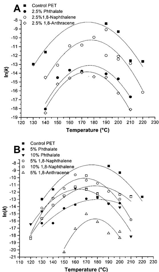
**Figure 6** Crystallization rate versus temperature: (A) 2.5 mol % copolymers; (B) 5 and 10 mol % copolymers.
