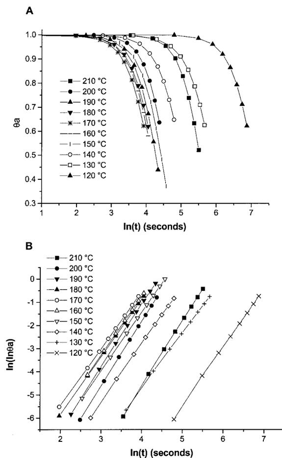
**Figure 5** Example of Avrami treatment of isothermal crystallization data for the 5 mol % 1,8-naphthalene copolymer: (A) Crystallization isotherms; (B) Avrami plot.
