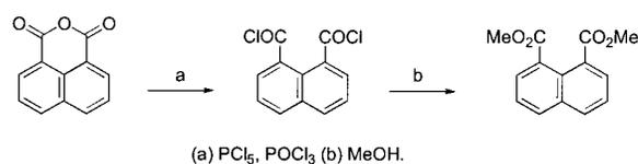
**Figure 3** Synthesis of dimethyl 1,8-naphthalenedicarboxylate.
