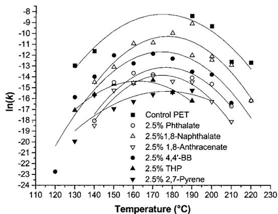
**Figure 7** Crystallization rate versus temperature for 2.5 mol % copolymers. Comparison of linear and U-turn copolymers.
